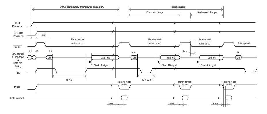
Figure 3: Timing diagram for STD-302
